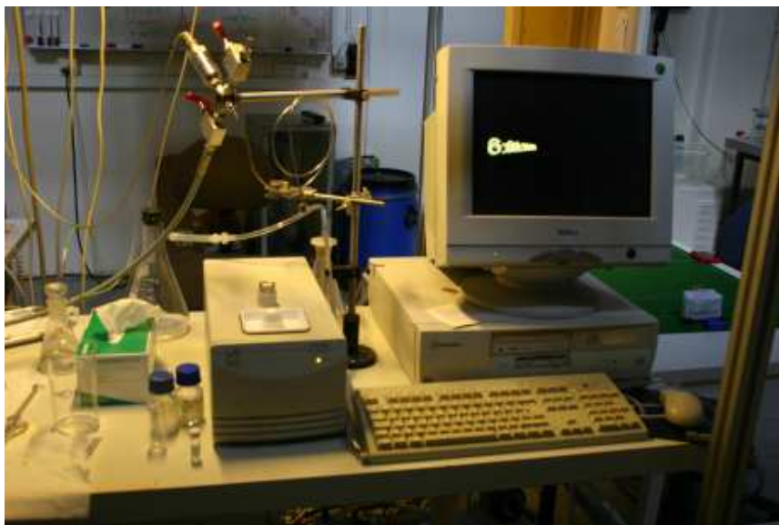
Figure 8: The used VP differential scanning calorimeter.
