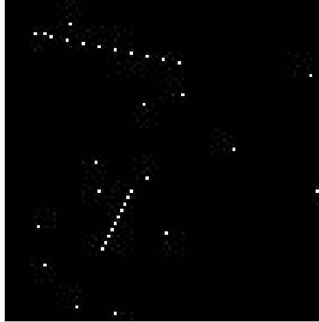
Figure 4.15: Image for test of the Hough transformation. It consist of 35 points in a 100 x 100 pixel image.
