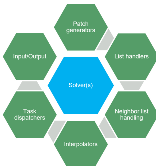
FIGURE 11. The architecture of the framework is such that the solvers sit in the middle and only handle the specific task of solving the physics in its given task area, everything else is then services functions around the solver. The solvers do not call any interface routines. Credit: Åke Nordlund
