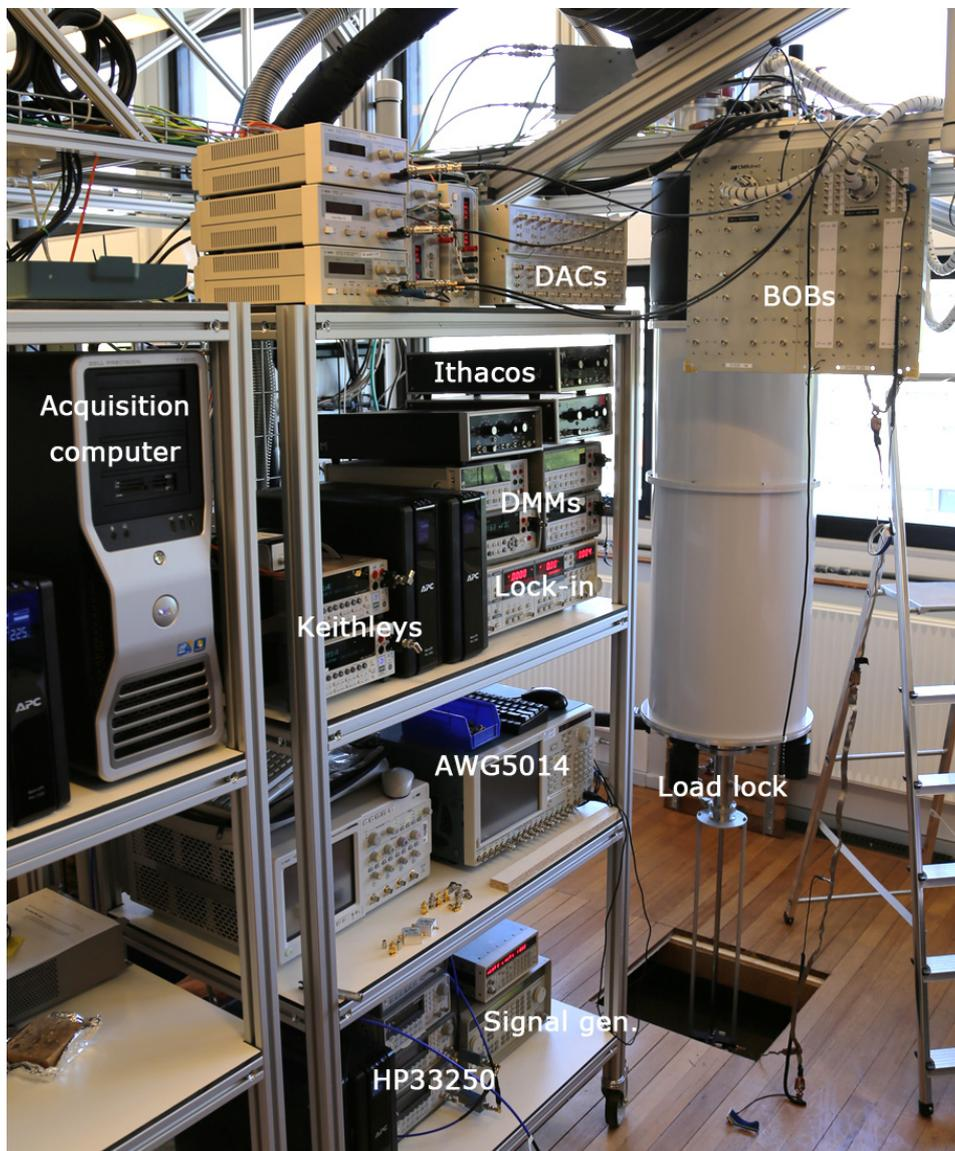
**Figure 3.11:** Image of the room-temperature electronic devices used in the experimental setup.
