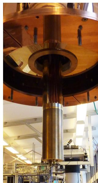
**Figure 3.9:** Sample puck loaded onto cold finger on cryostat with vector magnet off.
