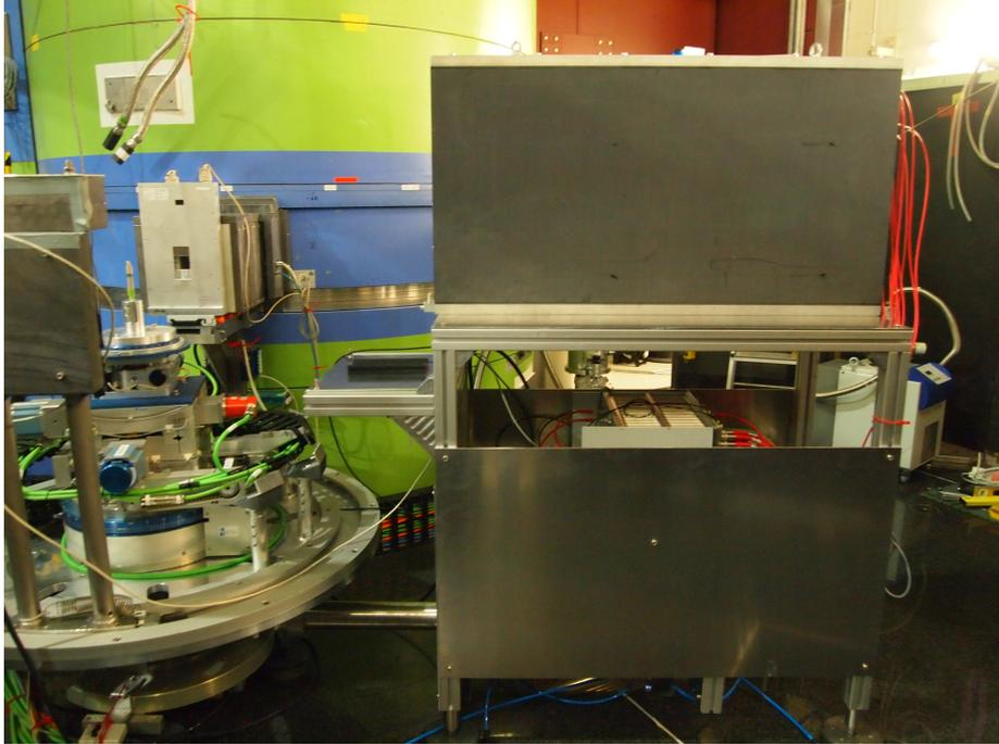
Figure 27: The MultiFLEXX prototype (grey rectangle upper right), mounted in the back-end position of the PANDA TAS via an aluminium tube (bottom center). Behind the metal plate (lower right) is the detector electronics. Left, we have the sample position and translation tables/tilt stages for the sample, along with the beam stop. The large green/blue/green cylinder in the background houses the monochromator.
