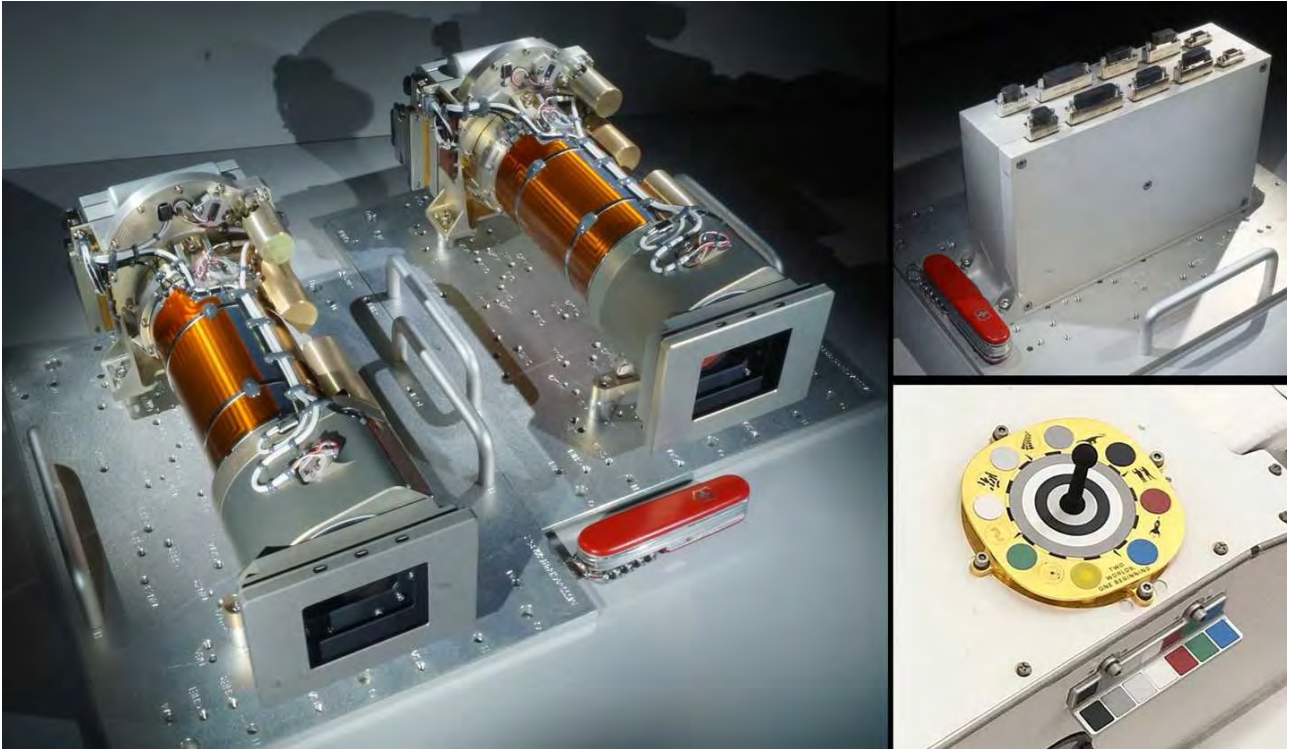
Fig. 3 - Overview of the Mastcam-Z components. (Left) Camera heads before mounting on the RSM. (Upper right) Digital Electronics Assembly (DEA) before mounting inside the rover chassis. (Lower right) Calibration targets mounted on the rover deck. For scale the pocket knife is 88.9 mm long, and the primary calibration target is 8 x 8 cm across. From: Bell et al., 2021
