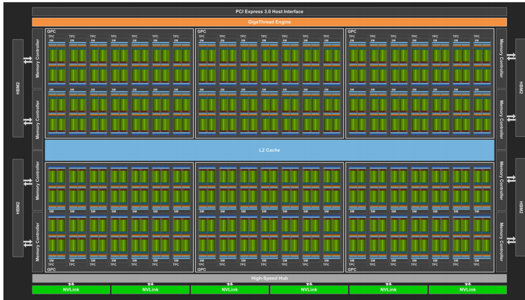
FIGURE 5.2: GPU achitecture (Dr. Momme Allalen, 2020)
