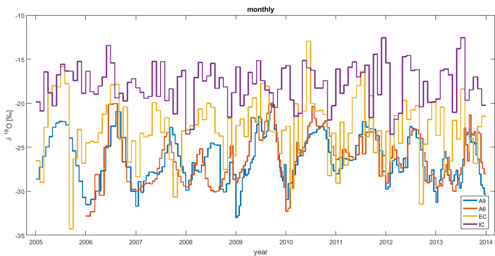
Figure 6.3: Monthly \delta^{18}\text{O} -values for 2006-2013, including, from both firn cores (A6 red and A9 blue) and models (ISOCAM purple and ECHAM yellow). For the firn cores, the temporal resolution is about monthly to bi-weekly.
