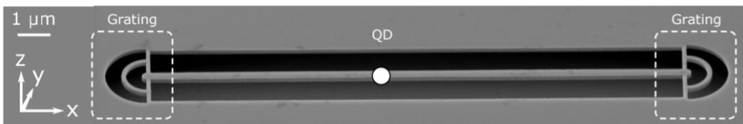
FIGURE 3.4: Scanning electron microscope image of a GaAs nanobeam waveguide embedded with a quantum dot and suspended in air. The gratings in the ends of the waveguide scatter light in the z-direction. Due to the high difference in refractive index between GaAs ( $n \sim 3.5$ ) and air ( $n \sim 1$ ) the mode of an emitted photon is confined to modes travelling along the waveguide. These modes are referred to as *waveguide modes*.
