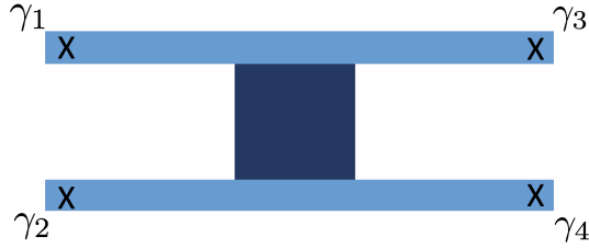
Figure 2: Sketch of the Majorana box qubit. Two nanowires are put on the same Coulomb blockaded island.
