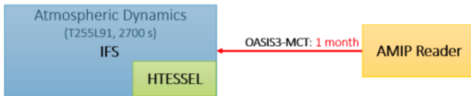
Figure 4.1: The IFS-standalone configuration in EC-Earth3 taken from Ludemann (2022). Within the IFS component, the standard resolution and accompanying time step are shown in blue parentheses. The supplement of oceanic observational data from AMIP to IFS through OASIS3-MCT is delineated by the red arrow.
