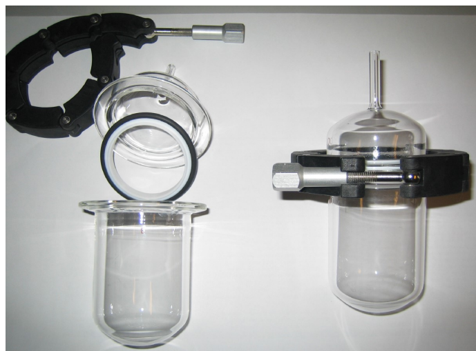
Figure 4.4: Photograph of glass extraction vessels along with their O-rings and connectors. Figure from Grzymala-Lubanski [2015].
