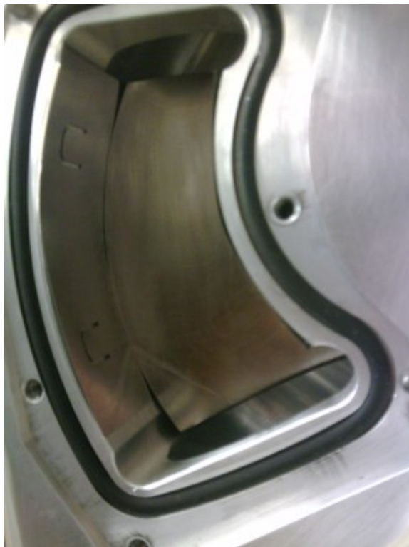
Figure 5.3: One of two shims placed between the magnet and the analyzer in the flight tube.
