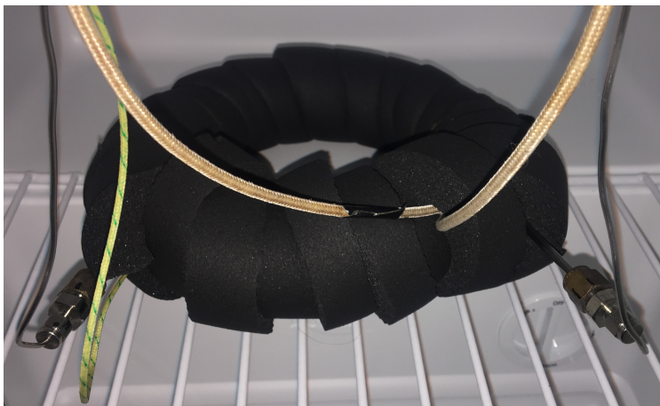
Figure 4.11: Picture of isolated GC column inside the freezer. The connection to the power supply for the heat tape is achieved by fitting the wires through holes drilled through the ceiling of the freezer.
