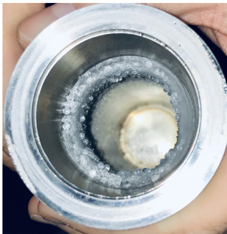
Figure 4.6: Inside of water trap, T1, after two samples have been melted and extracted. Water vapour freezes the glass beads along the walls.
