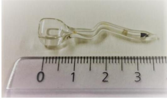
Figure 3: An example of a 5 mm cubic vapor cell [9].
