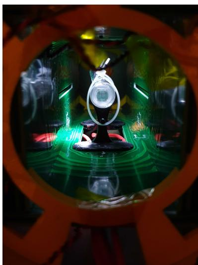
Figure 53: A picture of the inside of the magnetic shield where both the coil system and the 8 cm cell is mounted.
