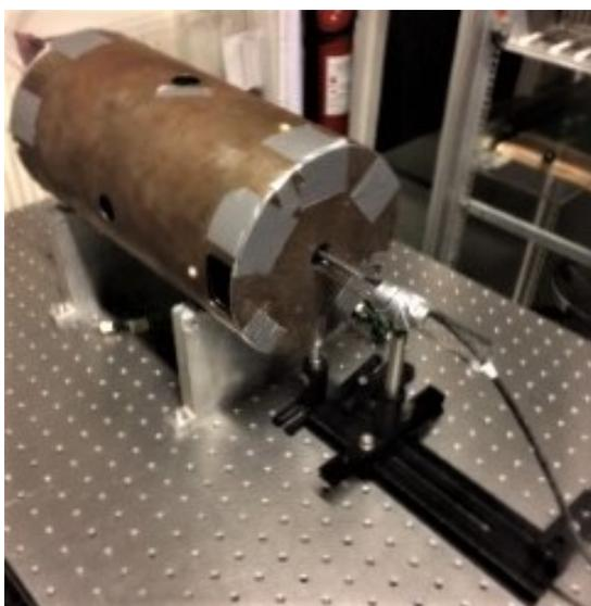
(b) Glass tube mounted on rails and USB probe inside the shield.
