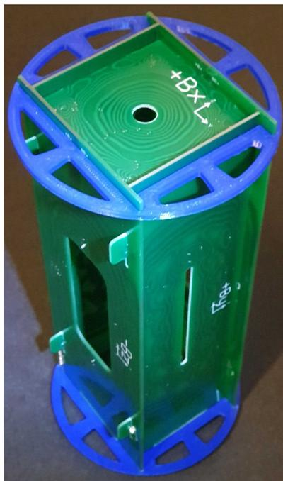
Figure 14: Picture of the assembled coil system.
