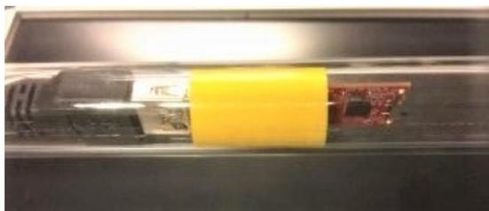
(a) USB probe mounted inside the glass tube.
