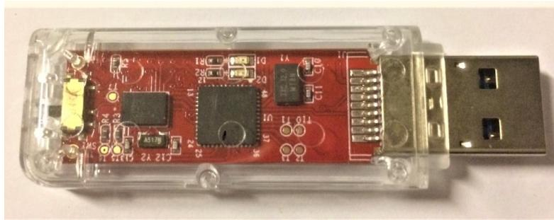
Figure 19: A *BNO055* USB probe used to perform magnetometry.
