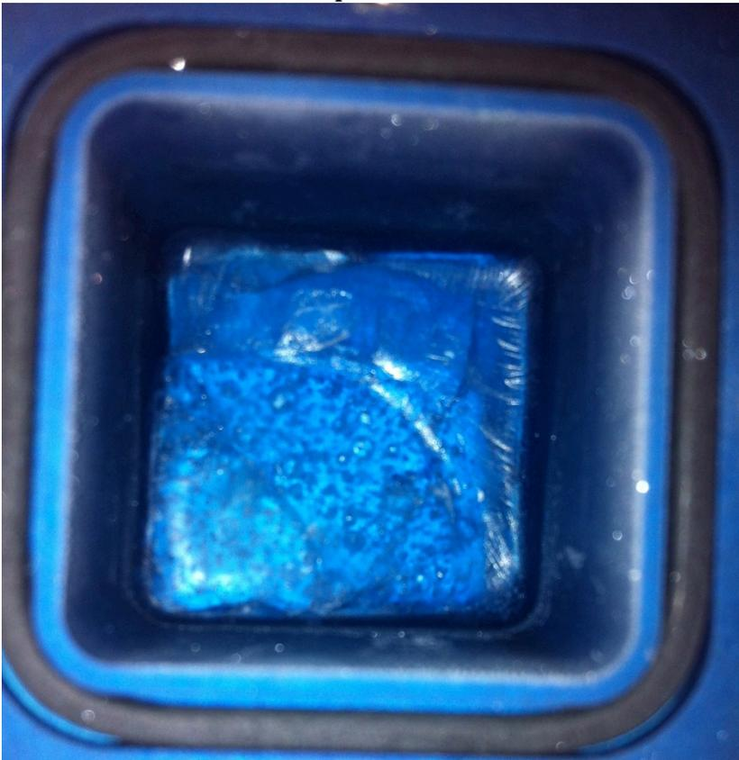
**Figur 65. The first sample after the measurement. Not all air was extracted; in the centre air bubbles are seen.**
