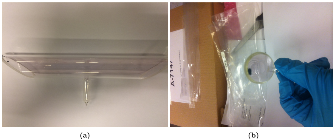
Figure 44: The iodine vapor cell. At room temperature the slight purple vapor is visible to the naked eye. (a) show the cell from the side and (b) show the end facet of the cell. The small dark looking granulate visible in (b) is solid state iodine.
