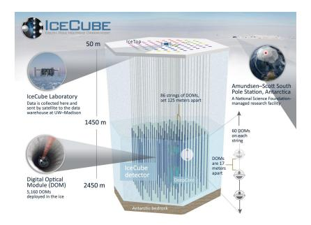
Figure 3: An illustration of the IceCube Neutrino Observatory. Shown is the main IceCube detector and the two subdetectors IceTop and DeepCore, and the IceCube Laboratory sitting on top of the detector. An illustration of the DOMs inside their borehole is also shown, with the number of strings, DOM spacing, and depth beneath the surface. Taken from Ref. [22].
