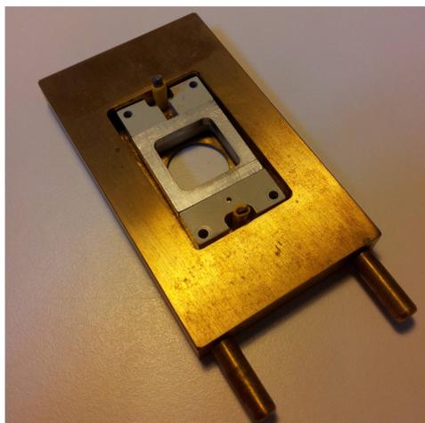
Figure 4.6: Experimental sample setup. The samples are attached to the inner plastic chamber from below, a square of metal is attached from above. Both have an electric connections to the electrodes sticking out. The chamber was screwed onto the brass block for stability and temperature regulation.
