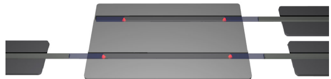
Figure 6.1: Illustration of a topological Kondo Effect setup. Graphical illustration of the simplest setup for detection of the topological Kondo Effect outlined by Béri and Cooper. In the middle, two parallel NWs are placed onto a superconducting Island. Three of the four NW ends are connected to normal leads and gates are used to tune the transport through the transparent parts of the NWs. A gate is meant to tune the levels of the island. At each part end of the NW-Island interface a Majorana state is formed giving rise to the topological Kondo Effect.
