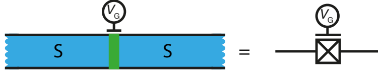
Figure 2.5: Two superconducting electrodes (blue) sandwiching a semiconductor (green) form a Josephson junction. The semiconductor is tuned by a nearby gate electrode making the Josephson junction gate tunable. On the right the circuit symbol of a gate tunable Josephson junction is shown.
