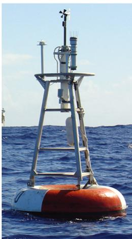
**Figure 3.1:** A picture of an ATLAS mooring positioned at sea. Modified from: NOAA (webA).
