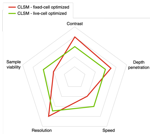
Figure 10: Illustration of how a CLSM instrument can be optimized to be more or less suitable for a particular experiment. Here, the trade off for five key parameters are shown for contrast vs. live-cell imaging. Adapted from Jonkman et al 69 .
