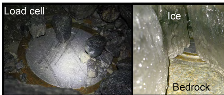
Figure 2.7: Two perspectives of the load cells the left image shows a plan view of the load cell. Note the striations on the metal surface of the load cell plate. The image right shows a side on view of the load cell with a column of 200m of overlying ice resting on the metal plate.
