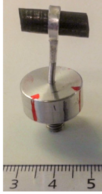
Figure 5.4.1: \text{La}_{1.93}\text{Sr}_{0.07}\text{CuO}_4 single crystal sample placed inside an aluminium sample holder. This is the exact configuration used throughout all the neutron scattering experiments.
