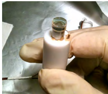
Figure 5.7.: Cavity mirror mounted on a piezo prior to mounting. The piezo is glued to a cylinder made of teflon with the optical axis free and a channel for the external wire for the piezo. The internal wire is glued to the inside of the optical channel.
