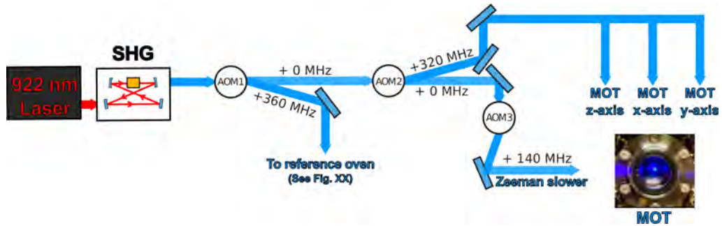
Figure 5.18: Overview of the detunings of the 461 nm cooling laser. AOM2 was used as a shutter for switching the MOT on and off in the experimental sequences. See Fig. 6.1c).
