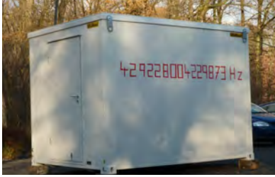
Figure 1.11: From [Riehle, 2015]: A picture of a transportable optical lattice clock, which fits inside a truck.
