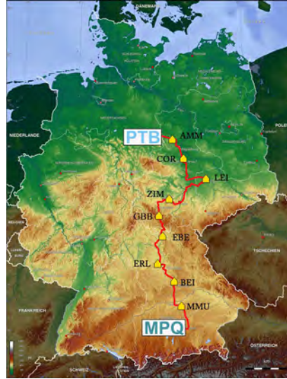
Figure 1.10: From [Predehl et al., 2012]: Map of a 920 km fiber link for frequency comparison realized between Munich and Braunschweig in Germany.
