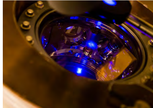
Figure 4.6: Picture of a MOT with trapped ^{88}\text{Sr} atoms. The bright blue spot is the fluorescence from the trapped atoms.
