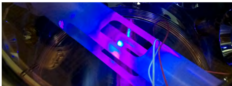
Figure 6.17: Picture of a MOT inside the cavity structure inside the main vacuum chamber. The fluorescence from the trapped atoms is seen as the central blue dot.
