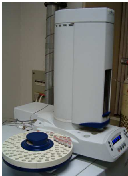
Figure 3.4: The Euro Vector liquid autosampler which is connected to the CF-IRMS. There are room for 110 samples in the rotating tray.
