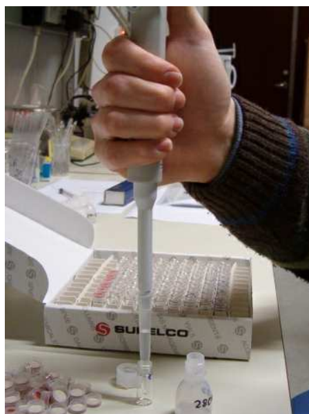
Figure 3.3: Samples were transferred from the airtight bottles to small septum-sealed vials, which could be penetrated by the syringe used by the autosampler.
