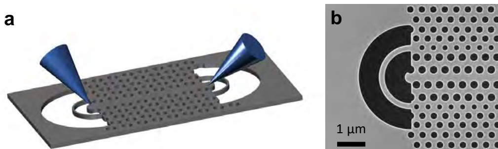
Figure 5.3: Schematic of probing technique. (a) An illustration of the angle of incidence and collection while exciting and measuring the transmission signal in a glide-symmetry waveguide resonator. (b) A scanning electron micrograph of a distorted circular grating coupler design caused by introducing glide-plane symmetry.
