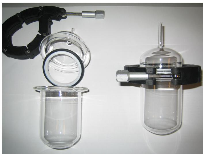
Figure 3.3 – The design of the extraction flask was chosen to minimize the volume of the extraction flask while keeping an easy access for ice samples. A bottom-rounded glass vessel was chosen to favor a higher exchange surface between the melt water and the headspace.
