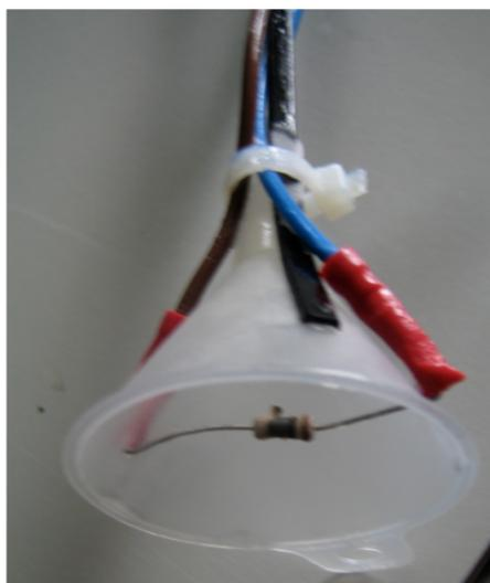
Figure 3.11 – An electric current passes through the  $10\ \Omega$  resistance immersed in a LN dewar. The hot heating element, thanks to the Leidenfrost phenomenon, enables LN droplets at  $-196^\circ\text{C}$  to be carried in their own vapour cushion through a plastic tubing at near ambient air temperature to the GC box without vaporizing within the tubing.
