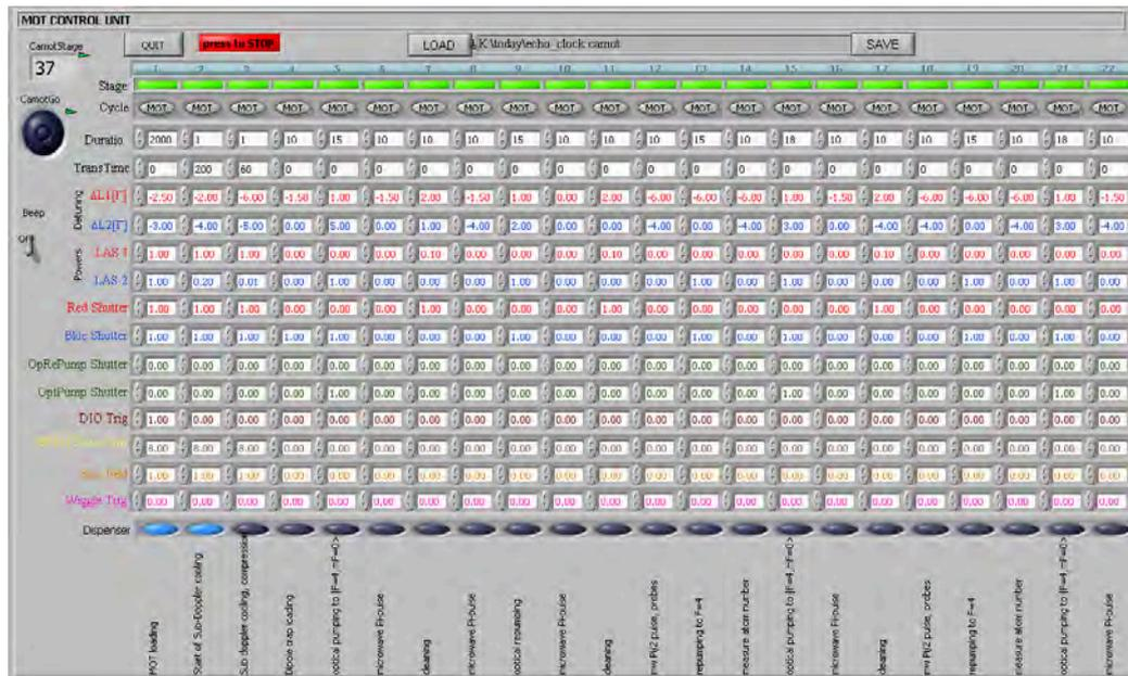
Figure 9.2: Screen-shot of a reasonably recent and representative version of the LabView programme CAMOT, which controls the National Instruments PCI cards and numerous other PC output busses.
