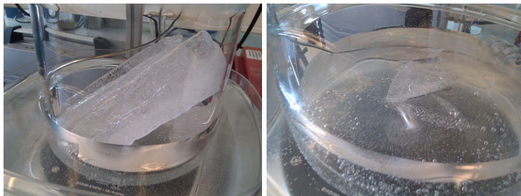
Figure 4.8: Left: Eurocore ice sample in the melting vessel. Notice the large groove in the sample. Right: Air bubbles resigning on the melting vessel walls.
