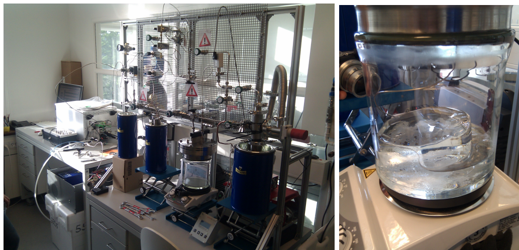
Figure 4.7: LEFT: Picture of the extraction system and CRDS analyzer. RIGHT: Picture of blank ice being melted in the melting vessel.
