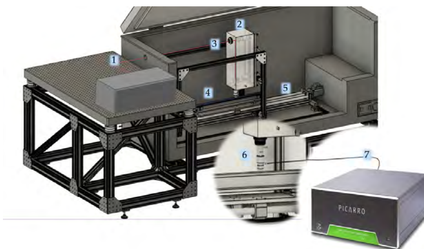
FIGURE 4.2: Laser ablation setup at the University of Copenhagen including high energy fs pulsed-Laser (1), reaching a mirror (2) mounted in the optical rail inside the freezer where a focusing system, enclosed in the cover box (3), directs the beam onto the ice surface placed in a holder (4), mounted on the linear translational stage (5). The ablation chamber (6) and the CRDS analyzer (7) serve for sample collection and water isotope analysis respectively.
