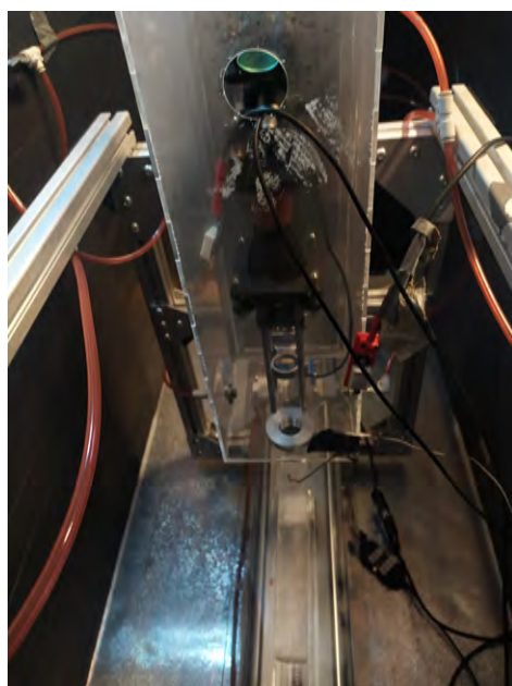
FIGURE 4.11: DHT22 sensors placed inside the optics enclosure and in the freezer area for monitoring humidity and temperature. Stainless steel tube interfacing the CRDS instrument is placed above the ice surface.
