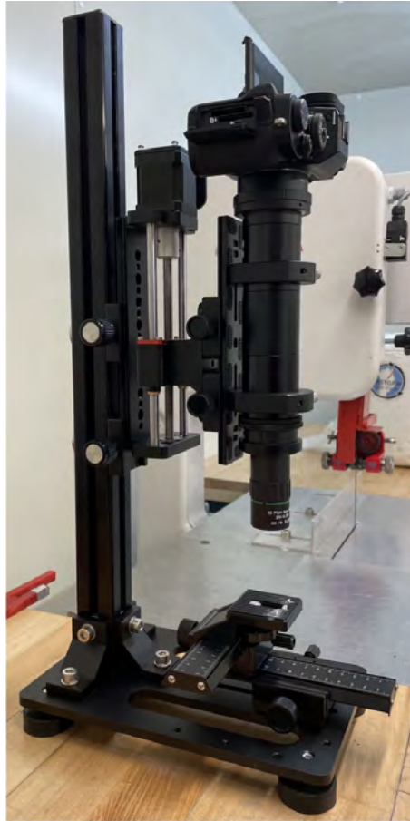
FIGURE 4.16: Macro-photography setup including motorized rail with a macro tube attached, mounted on a stand. The tube supports the camera at one end and the objective lens at the other. The stand incorporates a XY stage where the sample is placed.
