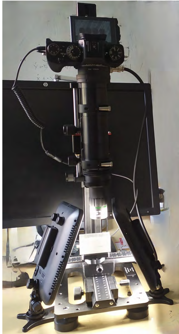
FIGURE C.1: Macro-photography system with LED panels lighting.
