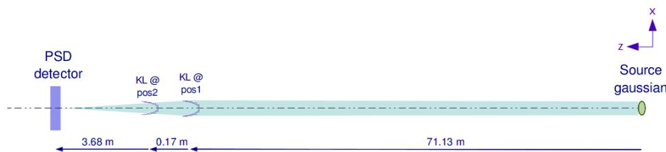
Figure 6.28: The simulation model implemented in McXtrace for the third series tests.
