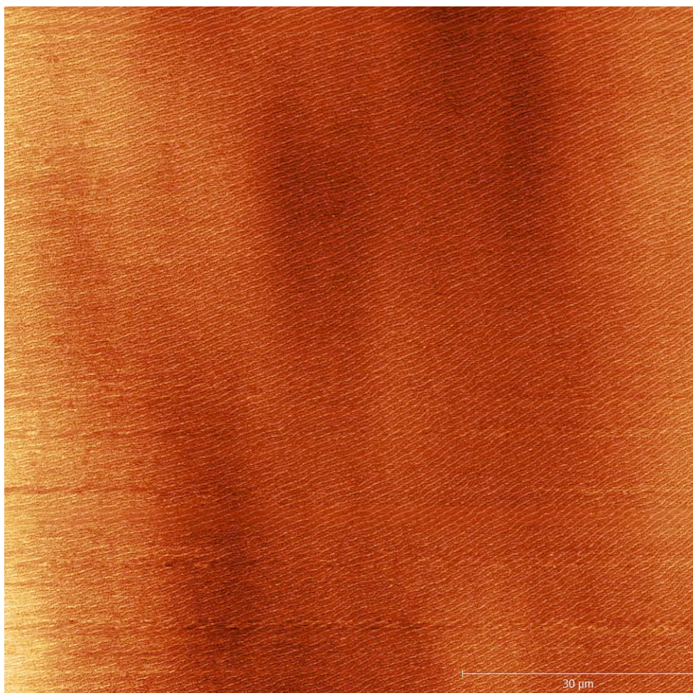
Figure 62: 90µm by 90µm AFM scan, showing that the stripe pattern covers huge areas with surprisingly few defects.
