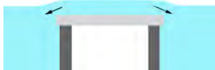
Figure 22. Visually assessing the level of water above the coverglass. Water drains slowly from the thin layer above the glass (arrows) this distorts the water surface. The thinner the layer and the faster the trough is drained the bigger the distortion. Experience with the specific trough and siphon allows a rather accurate and fast assessment. Dimensions of drawing are not to scale.
