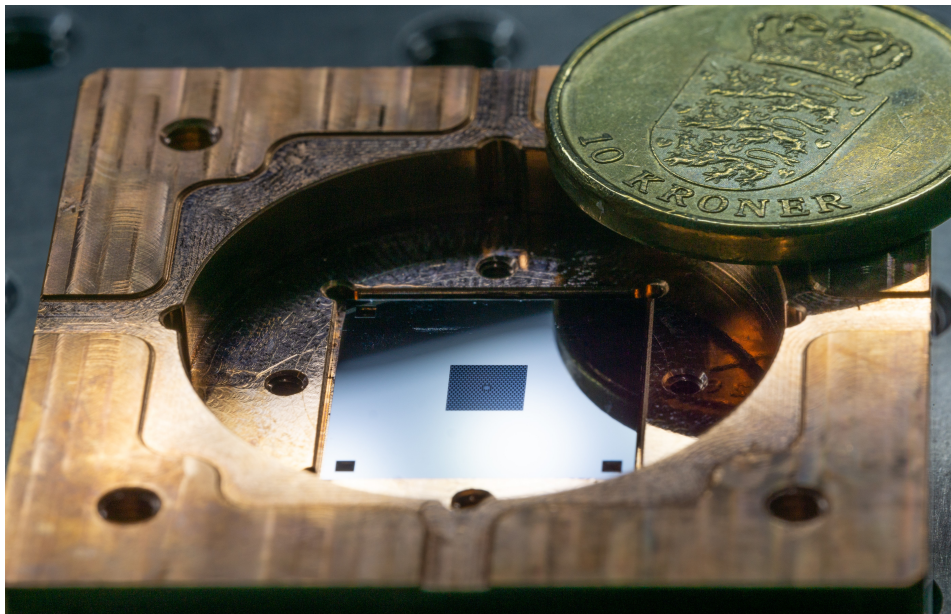
Figure 4.2: Photograph of a soft-clamped membrane resonator, lying in a sample holder for a cavity optomechanics experiment. The distance between the centers of the square alignment holes in the substrate is 15 mm. Photo courtesy of Julian Robinson-Tait.
