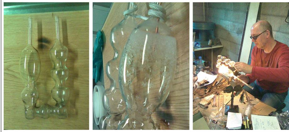
Figure 2.15: The equilibrium chamber is custom made (right) of several spheres to increase the ice-vapor exchange (left). When mounted in the cooling bath the parts above the liquid level are heated and the addition of an outlet tube results in the vapor condensing out below the liquid level (middle).
