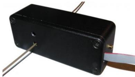
Figure 3.11: The internal and external part of the head stage with a tube passing through it. For this application the head stage is consisted of two measurement circuits, in which two solutions can be measured simultaneously. (EDAQ C4D website: http://www.edaq.com/product_sheets/transducers/ET125_General_Purpose_C4D_Headstage.pdf )
