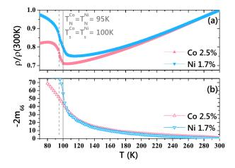
Figure 5.12: Comparison of elastoresistivity coefficients for Co and Ni doped samples with identical  $T_N$  values. T dependence of (a) the normalized resistance and (b) elastoresistivity coefficient  $-2m_{66} \propto -d\eta/d\epsilon$ . From [80].
