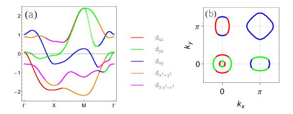
Figure 6.5: (a) Orbitally resolved band structure with  $\Gamma = (0,0)$ ,  $X = (\pi,0)$  and  $M = (\pi,\pi)$  denoting the symmetry points in the BZ corresponding to the one Fe unit cell. The main orbital contributions are shown by the colors as specified in the legend. (b) Fermi surface of the five orbital tight-binding Hamiltonian for the undoped system showing three hole pockets at  $\Gamma$  and M points and two electron pockets at X and Y points.
