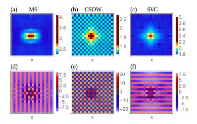
Figure 2.12: (a.c) Total (spin-summed) LDOS  $N(r, \omega = 0)$  around a  $V_p = 0.5$  eV non-magnetic impurity in the (a) MS, (b) CSDW, and (c) SVC states. (d)-(f) Local spin polarization percent  $P^l(\mathbf{r})[\%]$  of the corresponding cases in the upper row with l = y, z and x, respectively.
