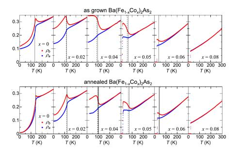
Figure 5.2: Temperature dependence of the in-plane resistivity (in m $\Omega$  cm units)  $\rho_a$  (blue) and  $\rho_b$  measured on detwinned (a) as-grown and (b) annealed Ba(Fe<sub>1-x</sub>Co<sub>x</sub>)<sub>2</sub>As<sub>2</sub> crystals. Vertical lines indicate  $T_s$  (solid) and  $T_N$  (dashed) under unstressed conditions. From [68].
