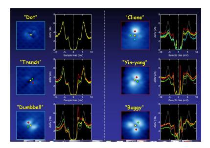
Figure 6.2: STM and STS measurements on native defects of LiFeAs. Some of the dI/dV spectra show clear in-gap bound states. From [119]
