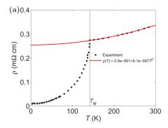
Figure 5.3: Dots: resistivity data extracted from Ref. [68]; line: fit to the data in the high temperature paramagnetic phase to  $\rho_{avg} = 2.5 \times 10^{-1} + 9.1 \times 10^{-7} T^2$ .
