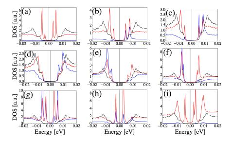
Figure 6.7: Total LDOS for nonmagnetic point-like scatterers at the impurity site (blue line) and at the NN site (red line). Panels (a-i) correspond to  $V_{\rm imp} = -8.0, -1.5, -0.75, -0.4, 0.4, 0.75, 1.5, 2.0, 8.0 \text{eV}$ . In all plots the solid black line is the DOS of the clean SC.
