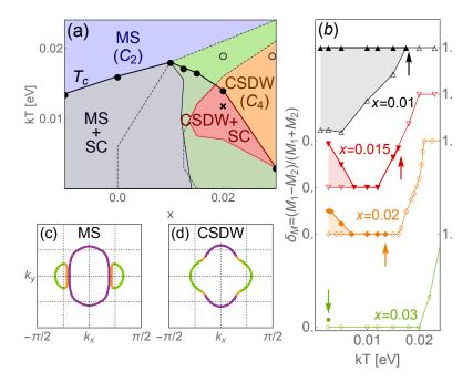
Figure 2.9: (a) Modified phase diagram from the region indicated by the dashed box in Fig. 2.4(e) in the presence of SC order. (b) Magnetic anisotropy  $\delta_M = (M_1 - M_2)/(M_1 + M_2)$  versus T for four different x with (without) SC order shown by the solid (open) symbols. The arrows mark  $T_c$ . (c,d) Fermi surface at the cross in (a) for MS (c) and CSDW (d) order (without SC) using the same orbital color code as in Fig. 2.6.
