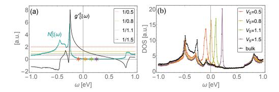
Figure 4.4: (a) Graphical solution of equation (4.6) for different  $d_{3z^2-r^2}$ -only impurity strengths  $V_5$  as specified in the legend. (b)  $N(\mathbf{r}, \omega)$  at the impurity site for the  $V_5$  cases used in (a). The total homogeneous DOS (black) is also shown as a reference.
