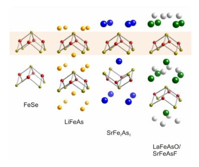
Figure 1.1: Crystallographic structures of various FeSC subfamilies. From left to right 11, 111, 122, 1111. From [2]
