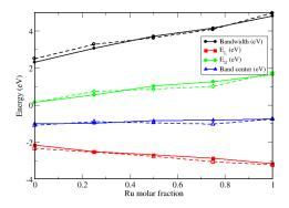
Figure E.2: Band parameters for TM related *d*-bands. Solid lines and filled symbols refer to  $LaFe_{1-x}Ru_xAsO$ , while dashed lines and open symbols refer to  $SmFe_{1-x}Ru_xAsO$ .
