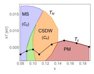
Figure 2.10: Phase diagram showing the magnetic and superconducting phases as a function of T and filling  $n_{opt} - x$  for U = 0.85 eV.
