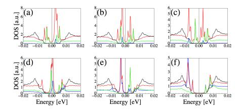
Figure 6.8: Total LDOS for magnetic point-like scatterers at the impurity site (blue lines) and at the NN site (red lines). The green lines show the spin-up LDOS at the NN site. Panels (a-f) correspond to  $V_{\rm imp} = -8.0, -6.0, -4.0, -2.0, -1.0, -0.5 {\rm eV}$ . Repulsive potentials lead to the same total LDOS (with interchanged spin polarization of the individual bound states).
