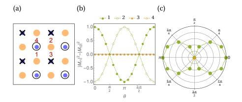
Figure 2.14: Difference between the moment amplitudes at the neighboring sites as a function of  $\theta$  (equation (2.13)) in the CSDW state. (a) Four inequivalent sites 1,2,3 and 4. (b)  $|\mathbf{M}_{r_1}|^2 - |\mathbf{M}_{r_2}|^2$  for the inequivalent sites as specified in (a). (f) Polar plot of the absolute value of the total change  $|\mathbf{M}_{r_1}|^2 - |\mathbf{M}_{r_2}|^2$  for sites 1 and 2 (green) and sites 3 and 4 (orange).  $\theta$  is illustrated in figure 2.13(a).
