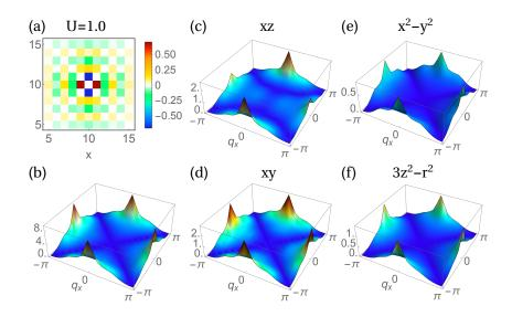
Figure 4.5: (a) Induced real-space magnetization in  $\mu_B$  around a  $V_{\mu}=6$  eV impurity, and (b) corresponding momentum space representation for U=1.0 and  $T/T_N=1.05$ . Orbital content  $m_{\mu}(\mathbf{q})$  for the  $t_{2g}$  orbitals (c) xz and (d) xy, and the  $e_g$  orbitals (e)  $x^2-y^2$  and (f)  $3z^2-r^2$ .
