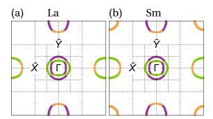
Figure 6.11: Fermi surface of (a) La-1111 and (b) Sm-1111. As the pnictogen height decreases (Sm  $\rightarrow$  La) the  $d_{xy}$  (orange)  $\gamma$  pocket disappears from the Fermi surface. The presence of this pocket is controlled by the nearest-neighbor  $d_{xy}$  hopping parameter,  $t_{xy}^{La} = 1.25t_{xy}^{Sm}$ .
