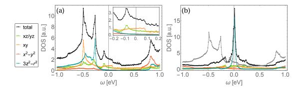
Figure 4.3: (a) Total DOS  $N_0(\omega)$  in the unperturbed normal state (black) and the contributions from the different orbitals as specified in the legend. Inset shows a zoom of 400 meV around  $\epsilon_F$ . (b) The same at the impurity site for the  $V_{\mu} = 1.1 \text{eV}$  and U = 0.3 eV case shown in figure 4.2. The unperturbed total DOS (gray) is shown for comparison.
