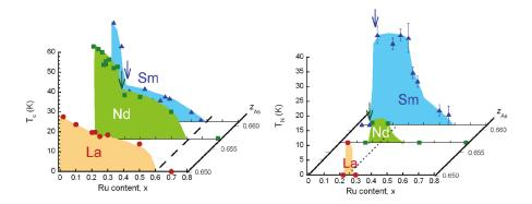
Figure 6.4: Transition temperatures in optimally doped  $L(\text{Fe}_{1-x}\text{Ru}_x)\text{AsO}_{1-y}\text{F}_y$  for L = La, Sm and Nd as a function of Ru content. (a) SC critical temperatures  $T_c$  and (b) magnetic ordering temperatures  $T_N$  from  $\mu$ SR measurements. From [137].
