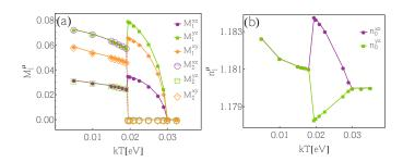
Figure A.1: Orbitally resolved (a) magnetic OPs for  $d_{xz}$ ,  $d_{yz}$  and  $d_{xy}$ , and (b) charge OPs for  $d_{xz}$  and  $d_{yz}$  as a function of temperature for x = -0.09.
