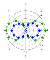
Figure 2.17: Spectral symmetry breaking parameter  $\delta_{C_2}(\omega = 0)$  as a function of  $\theta$  calculated at a magnetic site in the CSDW state (green), a non-magnetic site in the CSDW state (orange) and a site in the MS state (blue).
