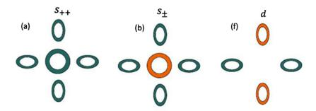
Figure 6.1: Schematic gaps  $\Delta_{\alpha}(\mathbf{k})$  of FeSC. Color represents phase the order parameter. From [106]
