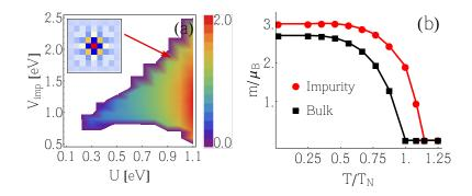
Figure 5.15: (a) Single impurity phase diagram displaying the impurity-induced magnetization at the impurity site at T=0 vs. U and  $V_{imp}$ . Inset: spatial magnetization of the induced impurity state at T=0 in the paramagnetic state. (b) Magnetization vs. T (normalized to the bulk Néel temperature  $T_N$ ) at the impurity site (red curve) and in the bulk (black) with U=1.6 eV ( $T_N=0.3 U$ ), and  $V_{imp}=0.1 \text{eV}$ .
