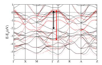
Figure E.1: Band structures for LaFeAsO (lines) and LaRuAsO (dots). The size of the dots is proportional to the weight of the Ru-4d orbitals. The LaRuAsO band structure is rescaled to fit the first Brillouin zone of LaFeAsO (see text).
