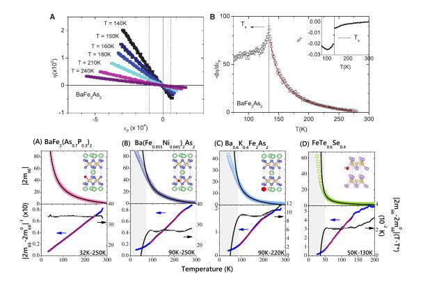
Figure 5.9: Elastoresistivity measurements. Top: (a) Relative change of resistivity  $\eta = \Delta \rho/\rho_0$  as a function of strain  $\epsilon = \Delta L/L$  at several temperatures above  $T_s$ . A linear fit of the data is shown in (b). The red line shows a fit to mean field model. From [66]. Bottom: Divergence of the elastoresistivy coefficient  $m_{66} \propto \eta$  (in absolute value) of several families in optimally doped Fe-based SC. From [81].
