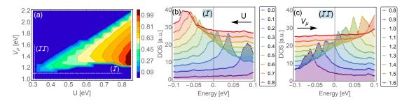
Figure 4.2: (a) Phase diagram of impurity-induced magnetization at the impurity site as a function of U and  $V_{\mu}$  in the normal state. (b) LDOS versus energy at the impurity site for  $V_{\mu} = 1.1$  eV varying U (path ( $\mathcal{I}$ ) in (a)), and (c) for U = 0.3eV and a representative range of potential strengths  $V_{\mu}$  (path ( $\mathcal{I}\mathcal{I}$ ) in (a)). Curves in (b) and (c) have been offset vertically for clarity.
