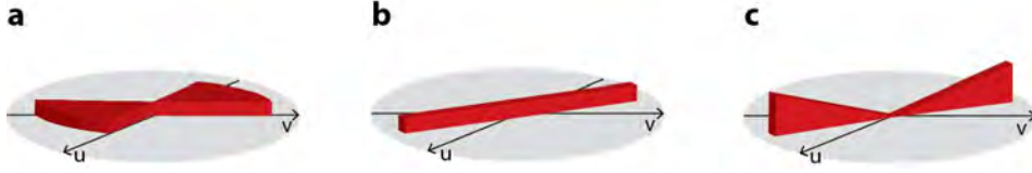
Figure 8.10: Schematic illustration of the Fourier transformation of the projections. a) The ideal case where the data covers a pie shape in Fourier domain and the object can be obtained by taking the inverse Fourier transform. b) Fourier transformation of a measured projection. c) In the Filtered Backprojection Algorithm a filter is applied to the data in (b) to approximate the situation in (a).
