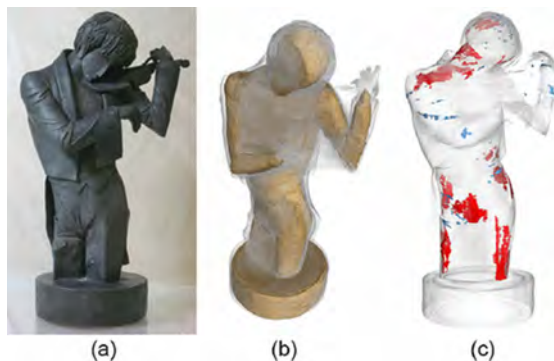
Figure 8.15: The lead and wood sculpture El violinista (1920) (a). 3D rendering of the wood core (b) and map of the areas (c) effected by corrosion (red) and needle fixations (blue) obtained by neutron tomography. Figure adopted from [79].
