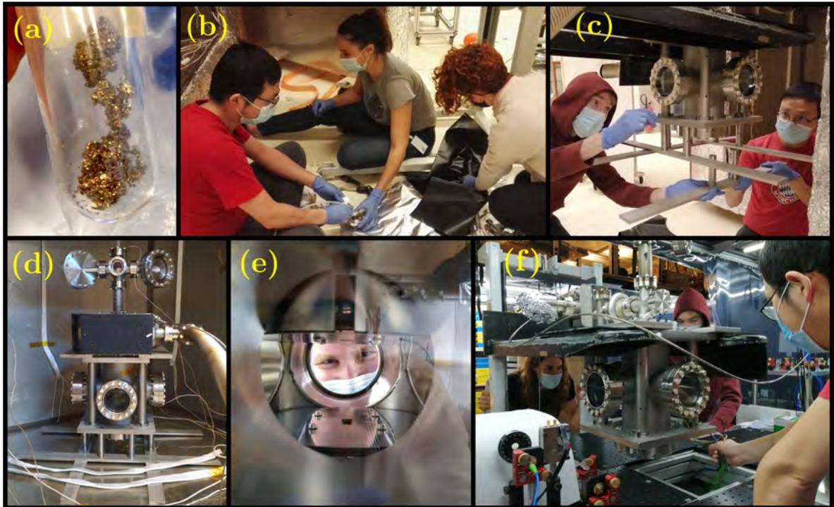
Figure 6.7: *Final assembly of the SRLM. (a) Strontium. (b) Loading strontium into the machine. (c) Preparing the machine for bake-out. (d) The machine within oven for baking. (e) The SRLM after assembly, lower part: heat shields and oven exit, center: Shayne, upper: science cavity. (f) Completion of oven connections and mounting onto breadboards.*
