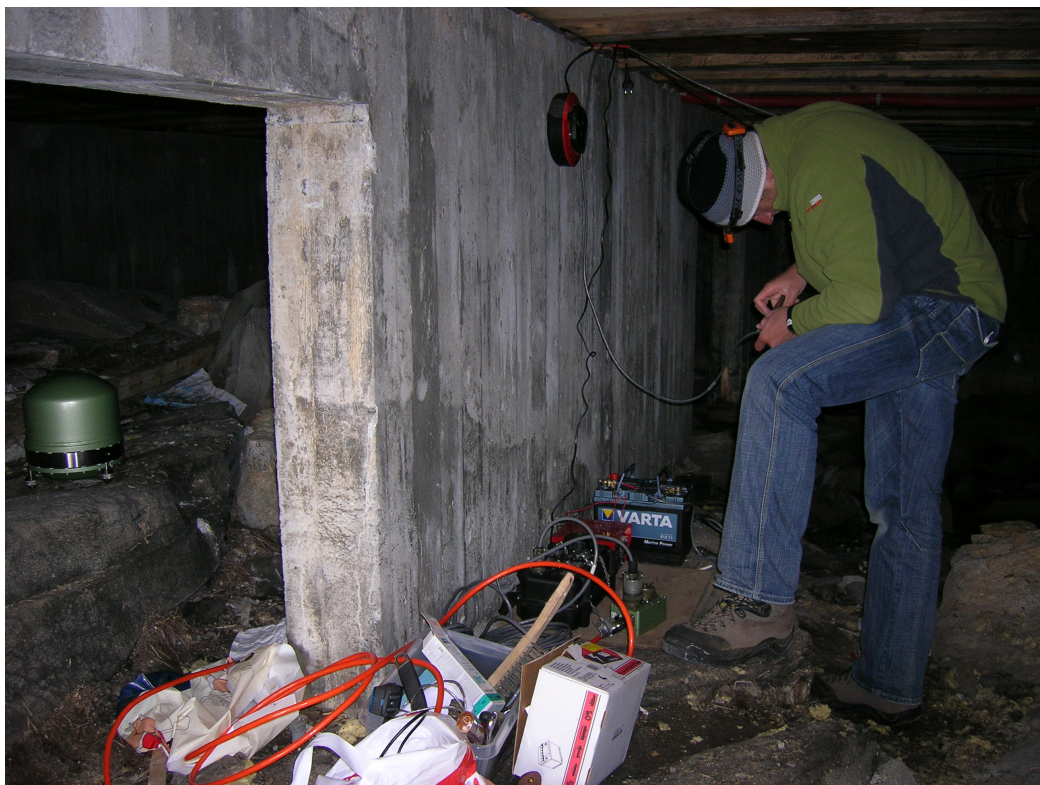
Figure 4.7: Installation of the seismometer in the settlement of Isertoq.
