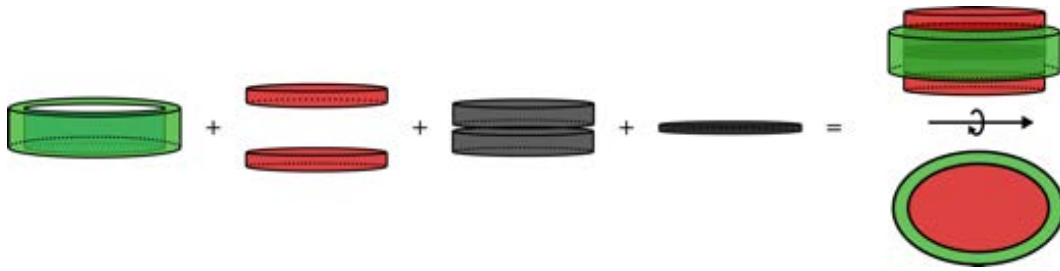
Figure 15 Geometric model of a nanodisc. The overall geometric model of a nanodisc is described by a hollow cylinder representing the MSP belt (green), two cylinders representing the lipid head groups (red), two cylinders representing the methylenes of the lipid tail groups (grey) and a cylinder representing the methyls of the lipid tail-groups. The cylinders are parameterized with an axis ratio that allows them to be elliptical, as seen from the top-view.
