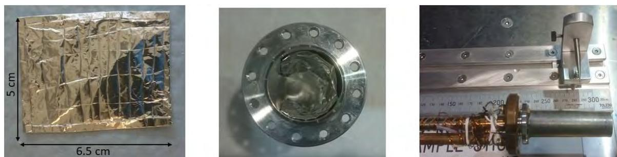
**Figure 30** Pictures of mounting process of the sample for the measurement at EMU.
