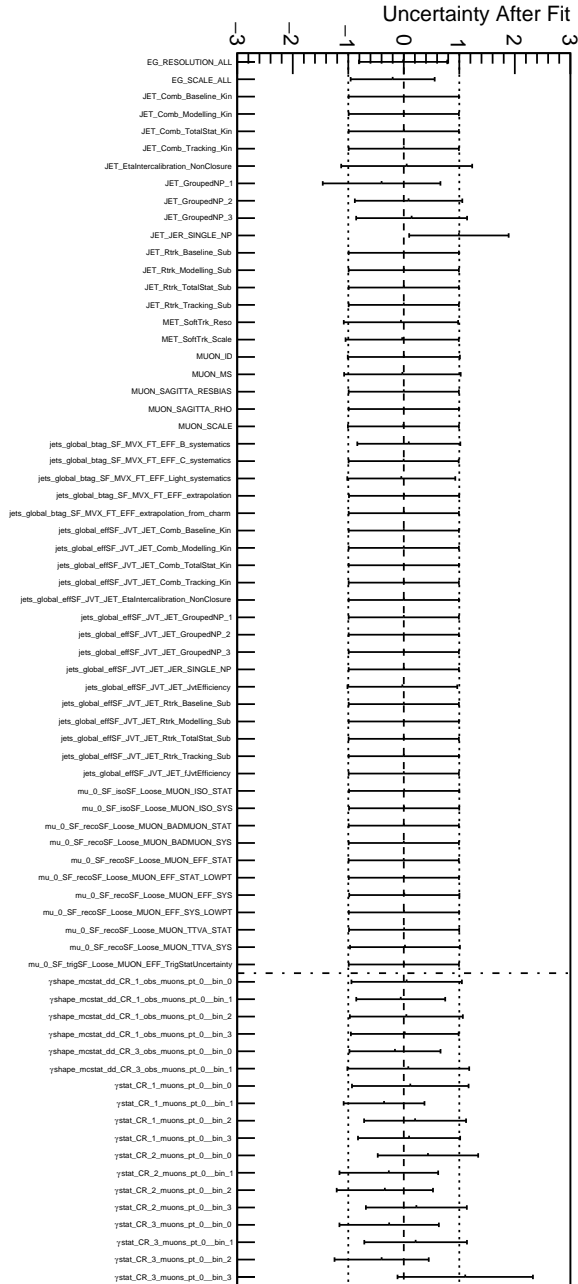
Figure 7.28.: Electron channel . Pulls of all parameters participating in the fit. The dataset is an Asimov dataset corresponding to the post-fit background-only model in the signal region and actual measured data in control regions.
