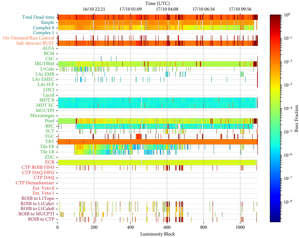
Figure 7.18: Busy summary for run 310738, showing the busy and dead-time fraction for each luminosity block for the various busy sources.
