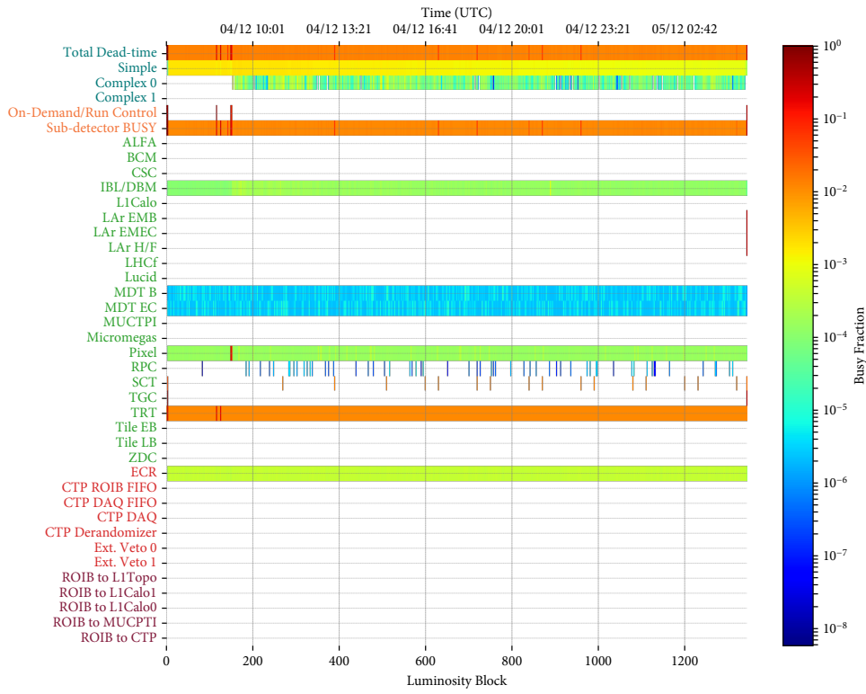
Figure 7.16: Busy summary for run 314199, showing the busy and dead-time fraction for each luminosity block for the various busy sources.
