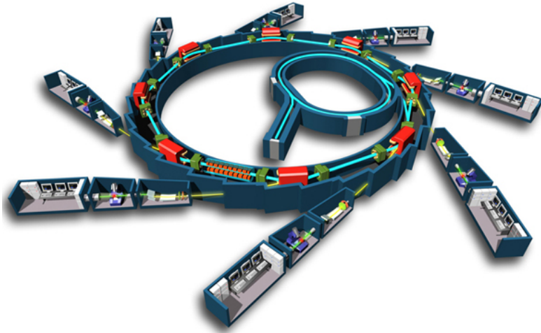
Figure 2.3: Outline on of a synchrotron facility (Soleil). A "short" linear accelerator called the linac accelerates electrons into a smaller ring called the booster ring. Here the electrons are further accelerated to near light speed and then injected to the storage ring. The different devises - bending magnets, wigglers and undulators produces the x-rays in the storage ring. In this illustration only bending magnets is illustrated to produce x-rays, however in theory every straight section of the storage ring could be swapped with an insertion devise. The produced x-rays are then transmitted into the beamline were the experiments are conducted. This figure is found via google search (Soleil 2019)
