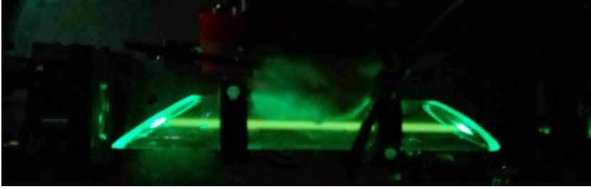
Figure 3.32: The iodine cell in a large waist cavity. The large TEM_{00} cavity mode is clearly visible as the iodine molecules fluoresce.
