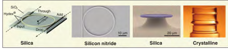
Figure 4.2: Examples of micro resonators used for frequency comb generation. From left to right: Silica waveguide ring resonator on chip [81], Silicon nitride waveguide ring resonator on chip [82], Silica toroid whispering gallery mode resonator [85],h and a crystalline millimeter-scale whispering gallery mode resonator [83]. Figure taken from [76].
