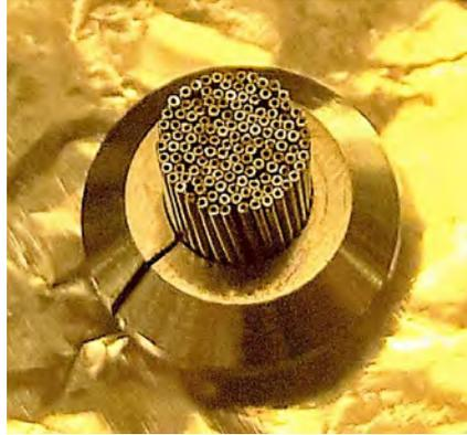
Figure A.1: Picture of the capillary tube holder for the Sr-2 oven, with tubes mounted.
