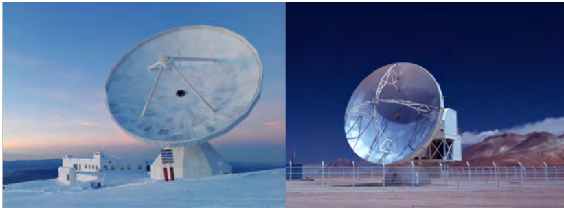
FIGURE 2.2 Examples of single-dish radio telescopes. IRAM 30 m telescope located at the Sierra Nevada Mountains in Spain (left; Credit: IRAM) and the APEX 12 m telescope located at the Chajnantor plateau in Chile (right; Credit: K.Zacher, ESO.).
