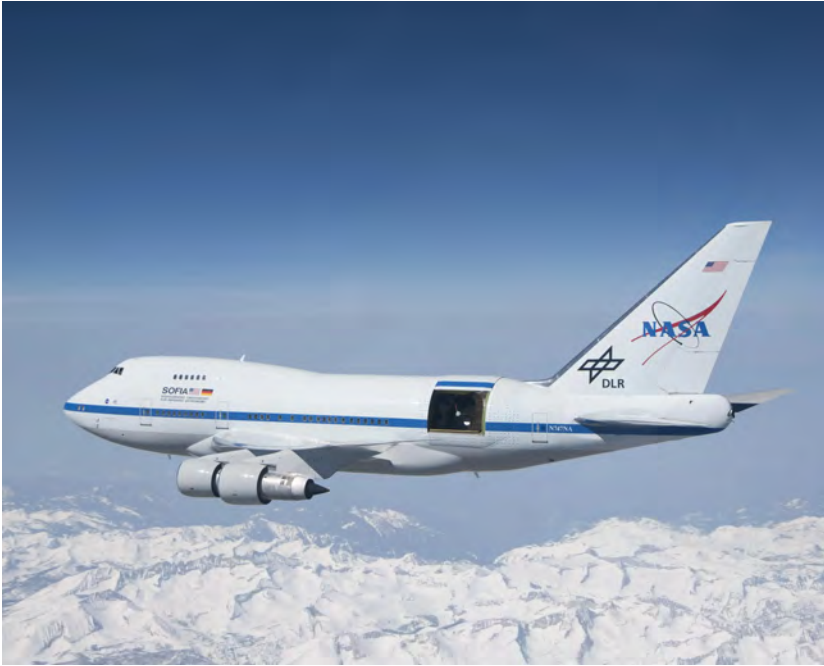
FIGURE 2.10 The SOFIA telescope in flight with its telescope cavity open for observation. Credit: NASA/Jim Ross.
