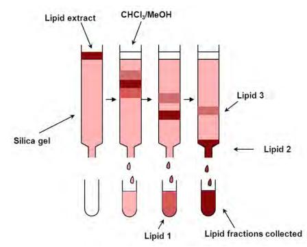
**Figure 4.3.** Phospholipid separation scheme. Silica gel chromatography set-up for separation of phospholipids according to head-group polarity. For details see text.
