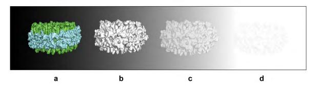
**Figure 2.1.** Schematic representation of the stealth nanodisc in a buffer solution with a gradually increasing level of  $D_2O$  (decreasing grayscale). (a) Hydrogenated nanodisc consisting of a phospholipid bilayer (green) and membrane scaffold protein MSP (light blue). (b) Stealth nanodisc comprised of deuterated lipid and deuterated MSP at 60% D2O. (c) Stealth nanodisc at 80%  $D_2O$ . (d) Stealth nanodisc at 100%  $D_2O$ .
