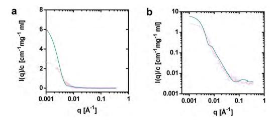
**Figure 6.8.** Stealth Liposome Performance. (a) Stealth liposome SANS data (light purple) and theoretical SANS data calculated for liposomes with commercially available  $D_{64}$ -POPC (Avanti Polar Lipids) (petrol). (b) A comparison of the two versions of deuterated liposomes (light purple and dark cyan) on a logarithmic scale.
