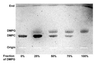
**Figure 4.8.** Separation of zwitterionic and charged lipids from nanodisc samples. After extraction lipids were separated on a TLC plate developed in chloroform/acetone/methanol/acetic acid/water (30:40:10:10:5 v/v/v/v/v). Lipids were visualised by primuline staining with 1,2-dimyristoyl-*sn*-glycero-3-phosphocholine (DMPC) and 1,2-dimyristoyl-*sn*-glycero-3-phosphoglycerol (DMPG) indicated on the left.
