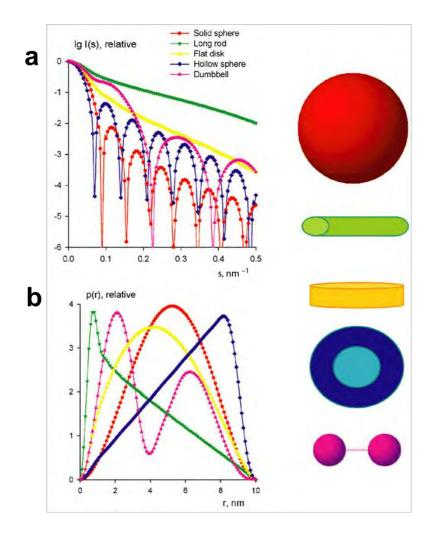
**Figure 1.7.** Scattering intensities and distance distributions of geometrical bodies according to Svergun and Koch<sup>123</sup> (2003). (a) Scattering intensity patterns for some typical geometrical shapes of the same size. (b) The pair distance distribution function P(r) for the shapes above after Fourier transformation.  $\bigcirc$  IOP Publishing. Reproduced by permission of IOP Publishing. All rights reserved
