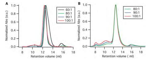
**Fig. 2** Size exclusion chromatograms of (A) pure DMPC and (B)  $X_{DMPA} = 0.25$  nanodiscs prepared at different DMPC to MSP1D1 ratios indicated in the figure label. Nanodiscs eluted at V = 12.3-12.6 ml, while lipid free proteins eluted at V = 16 ml and other lipid–protein aggregates eluted at V = 8-11 ml.
