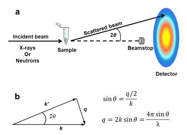
Figure 1.6. (a) Schematic representation of a small-angle neutron scattering experimental set up. A highly collimated neutron or X-ray beam illuminates the sample and the scattered radiation is recorded on a 2D detector. The beamstop absorbs the direct beam. (b) Scattering triangle for elastic scattering in which the incoming beam is deflected but does not gain or lose energy, |k'| = |k|.
