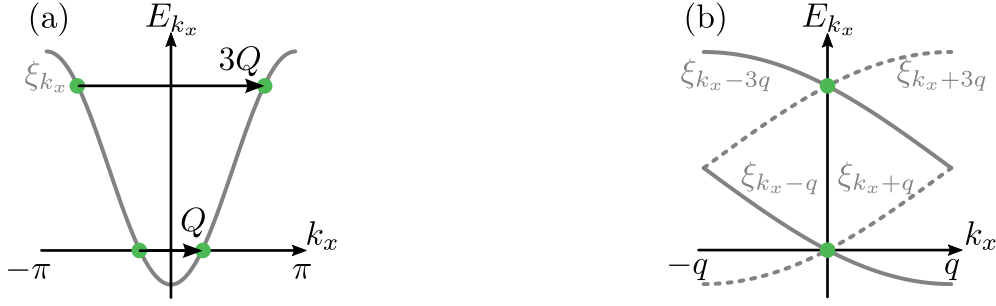
Figure 5.4: Example of a one-band model in 1D, obtained by considering a nearest neighbor hopping with strength t and a chemical potential value \mu_0 = -\sqrt{2}t < 0 . (a) The resulting dispersion \xi_{k_x} = -2t \cos k_x - \mu_0 contains two Fermi points at k_x = \pm\pi/4 of the 1 st BZ, which are connected by Q_N = Q = \pi/2 \equiv -3\pi/2 = -3Q . The texture also mediates the scattering between two points lying at E = 2|\mu_0| . (b) The resulting four bands of the dispersion in the MBZ. The points connected by the magnetic wave vectors are depicted with green dots.
